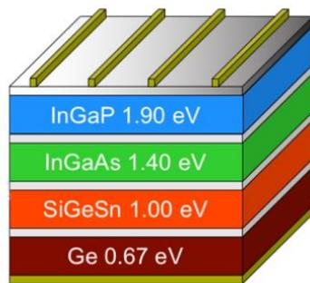
Figure 1: architecture of a four-junction solar cell using SiGeSn. From [2].
