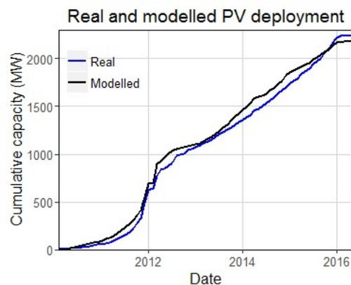
Figure 1: Real and modelled cumulative capacity of domestic PV installations with capacity less than 10 kW in Great Britain, after model calibration.
