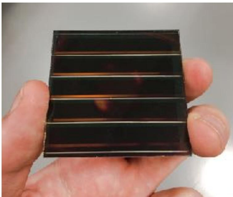
Figure 1. A series-connected perovskite sub module processed in a high humidity, ambient environment with a PCE of 11.8% over an active area of  $13.5 \text{ cm}^2$
